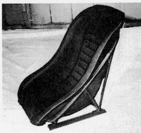
Anatomic racing seat. Steel tube supported plastic shell. Covered in matte black nap. From 33, used in GTA, GTA Jr., GTAm Wt. 6.6 lbs.
